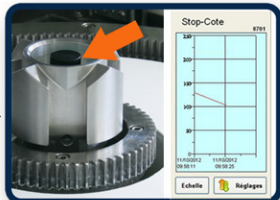
Automatic stop-on-size control system, measurement contactlessly and without wear
